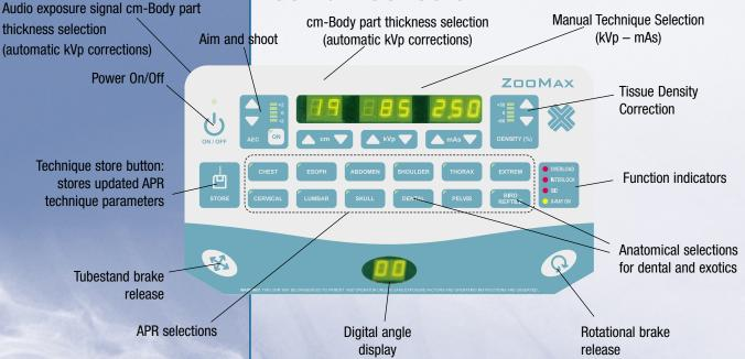
Integrated ZooMax HF generator control on the handlebar Veterinary Anatomical Programs are standard with the White system The generator can be installed in the table or can be separately mounted on the wall.
